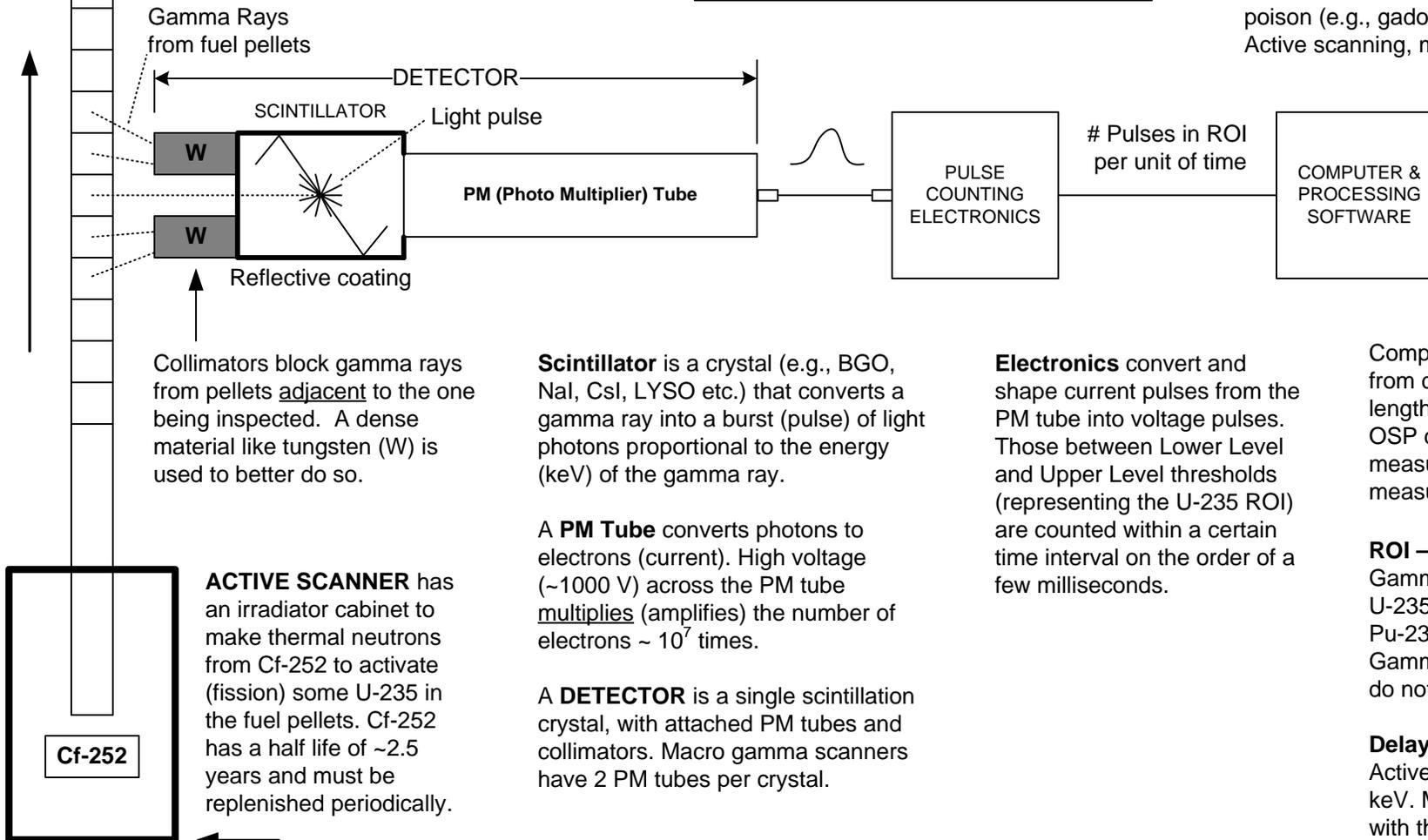
Collimators block gamma rays from pellets adjacent to the one being inspected. A dense material like tungsten (W) is used to better do so.
